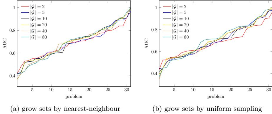
Fig. 2: Figures show AUCs of anomaly detection by LOFs, operating on subspace spanned by features used to explain anomalies identified by baseline LOF, for different grow set sizes. Explainer used for results in Left and Right figures utilized nearest-neighbour and uniform sampling grow sets respectively.
