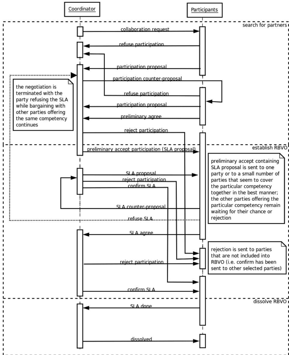
Figure 7 RBVO Formation Protocol hybrid state diagram (see online version for colours)
