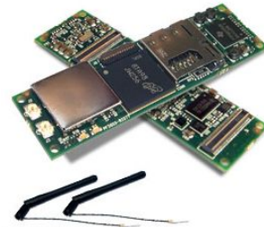
Fig. 4. On-board computer Gumstix Overo Fire.
