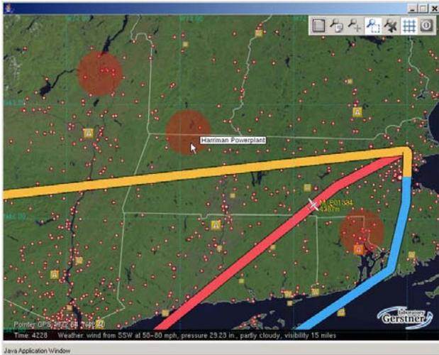
Figure 13: Flight plans avoiding no-flight zones
